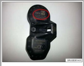
If P/N 4 078 787 or 4 079 152 is found, replace all four wheel electronics with P/N 36 10 6 856 227. If P/N 4 078 787 or 4 079 152 is **NOT** found, proceed as instructed by the ISTA test module and replace the indicated sensor.
