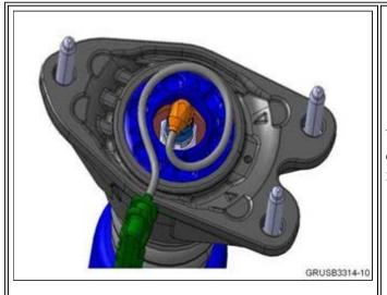
When positioning the connecting cable on the new shock absorber, both cables must be in one line.
