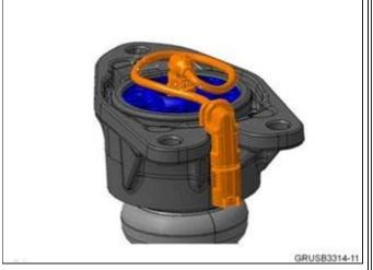
Turn both plugs in the installed position. Push them down until they snap into place.
