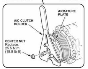
Using the A/C clutch holder from the A/C Compressor Kit, T/N 07AAF-000A150, remove the center armature plate nut. For more information about removing the A/C compressor clutch, refer to the *Tech2Tech* segment titled "Safely Remove That Rotor Pulley with the A/C Compressor Kit." 8. Remove the armature plate and the shim(s). Save the shim(s) to use as a baseline when assembling the new clutch parts.
