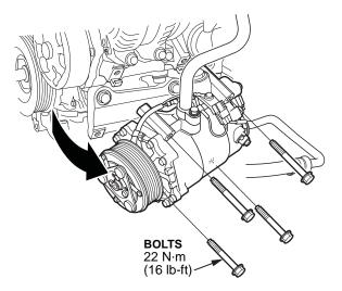
6. Carefully angle the compressor as shown below to support the compressor and take the stress off of the A/C lines.
