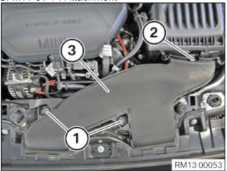
Remove the intake duct:
