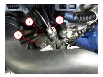
Install the auxiliary water pump:
