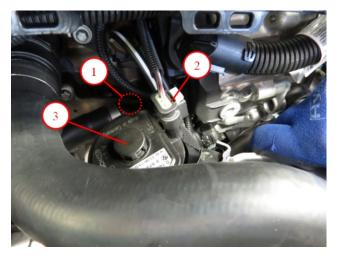
Release and remove the connection (1).
