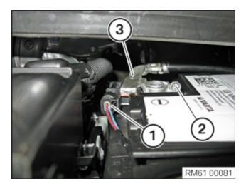
Unlock and disconnect the connector (1).
