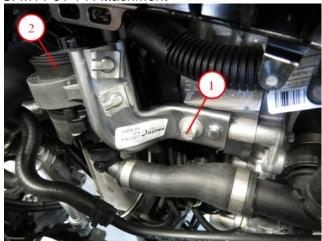
Clip the wiring harness (1) back together.
