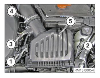
Install the intake silencer and intake duct:
