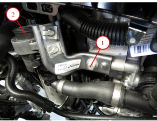
Remove the auxiliary water pump:
