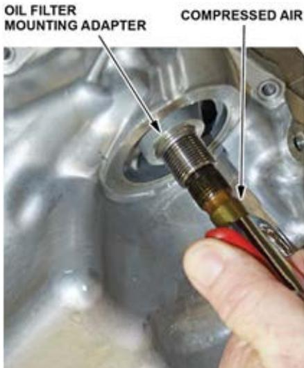
10. Blow compressed air for 5 seconds through the oil passage to clear any debris before installing the new cam chain auto-tensioner.
