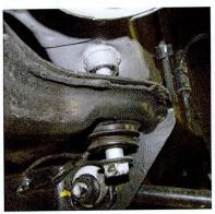
8. Use a pry bar to pull the subframe downwards slightly to create enough clearance between the control arm bolt and the fuel tank. Remove the bolt, and the right side rear lower control arm.
