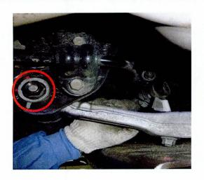
6a. If the control arm bolt(s) or other fasteners are difficult to remove, it may be necessary to cut the bolt(s) to remove the control arm.
