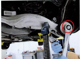
5. Carefully lower the transmission jack until the control arm swings down and releases the coil spring. Remove the coil spring.
