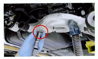
4. Remove the lower control arm bolt at the wheel side.
