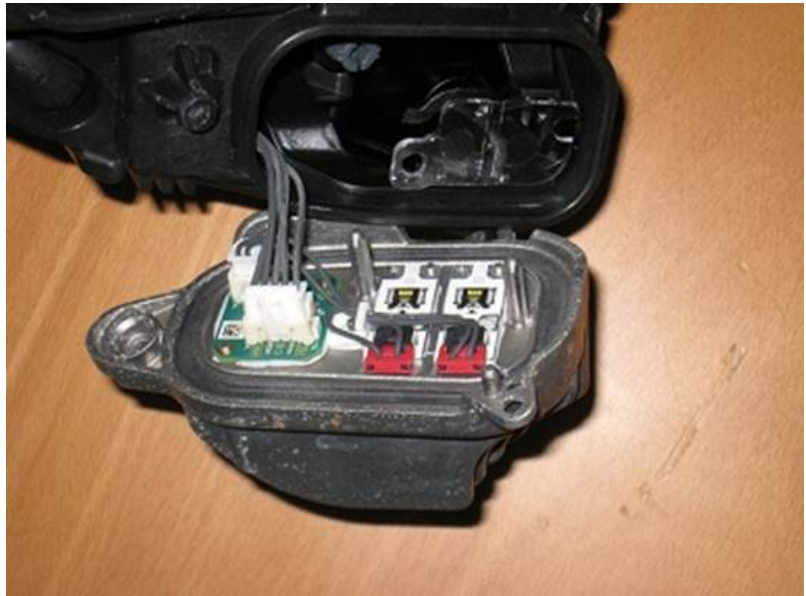
Figure 7: Dual surface mount LED unit exposed.
