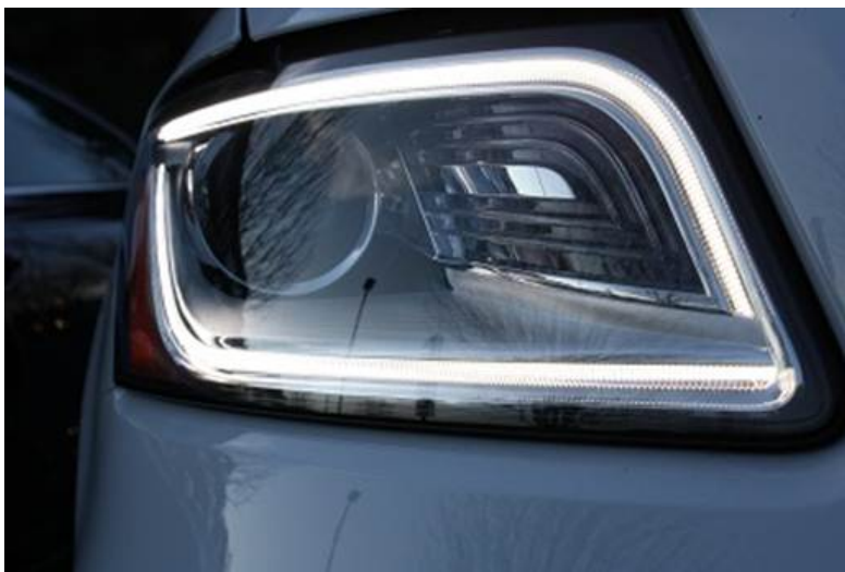
Figure 1. Upper and Lower light pipes illuminated.
