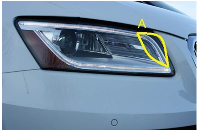
Figure 5. Upper light pipe perceived defect (A).
