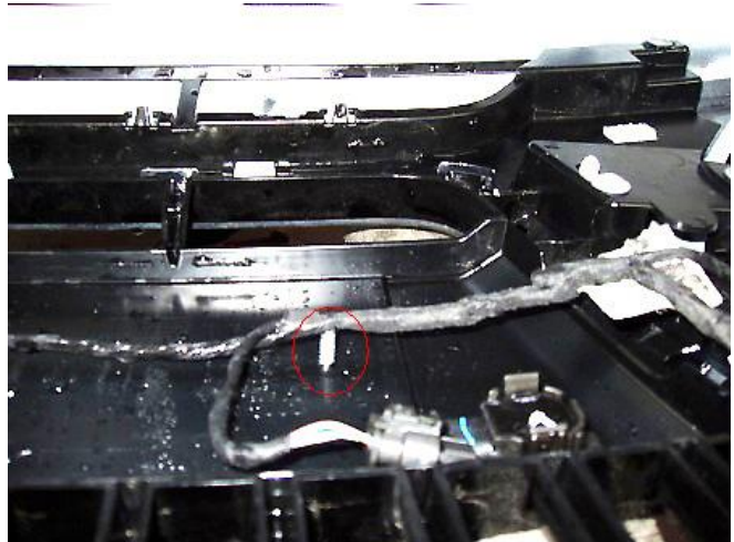
Figure 1. Damage to the wire harness for the parking aid system.
