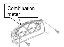
4. Render the old combination meter unusable by breaking the electrical connectors.
