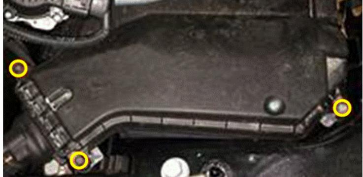
**Figure 4.** Screws to be removed (outlined).
