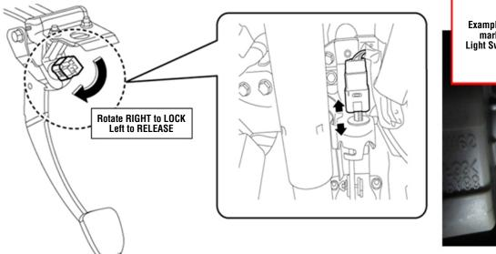
Example of the reference mark and the Brake Light Switch re-positioned 2 notches.
