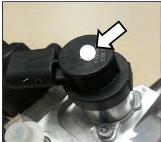
Figure 6. White dot on N290 fuel metering valve.
