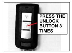
f. Within 10 seconds of completing Step 8e, press the unlock button on the F.A.S.T. Key 3 times. The door locks will automatically lock and unlock once, and then lock and unlock again after several seconds.
