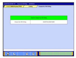
m. The Results of Chassis No./VIN Writing will display. Ensure the VIN is correct.
