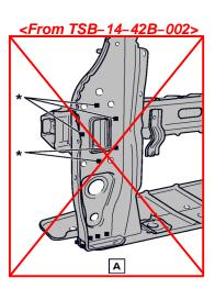
NOTE: \*: indicates the welding points of maker joint. (It is not necessary for repair)
