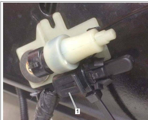
Fig. 2, New Ambient Air Temperature Sensor, Installed
