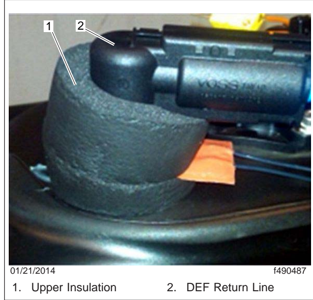
Fig. 3, Installing the Upper Half of the Insulation
