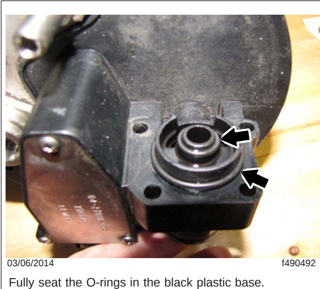
Fig. 6, Installing the O-rings
