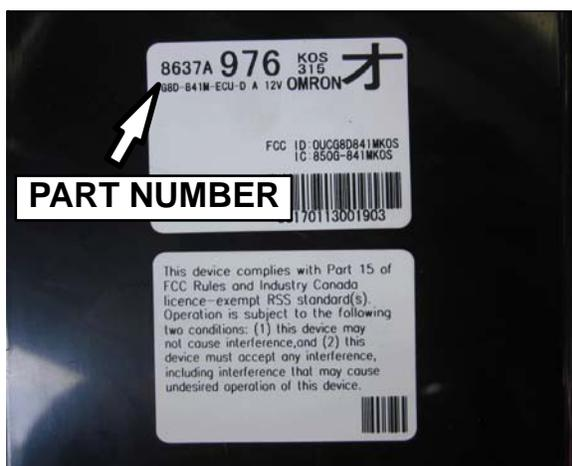
8. **Ensure the correct replacement KOS ECU part number is used. Please reference the Parts Information section for more information.** Install the replacement KOS ECU, (2) screws, and re-connect (2) connectors.
