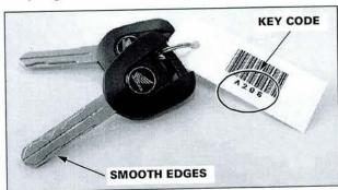
Available in automobiles for many years, the wave type key offers some distinct advantages over the conventional serrated-edge style keys such as much easier insertion and removal from lock cylinders. Also, wave type lock cylinders are much harder to defeat (pick) than serrated edge key types.
