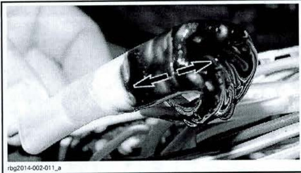
TYPICAL LIQUID TAPE APPLICATION
