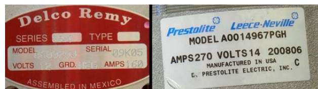
Fig. 6, Rated amps can be found on the label.
