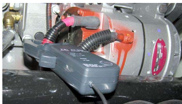
Fig. 13, Use an amp clamp around the positive alternator cable to measure the draw of the carbon pile.
