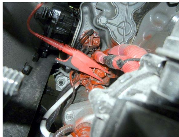
Fig. 8, Location of the starter positive post.
