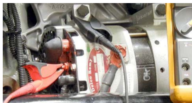
Fig. 14, Clip the DMM positive to the remote sense post and the DMM negative to the alternator body.
