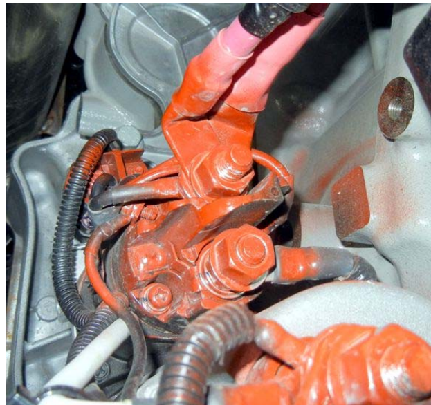
Fig. 10, Check the positive post on the starter solenoid for loose cables and corrosion.
