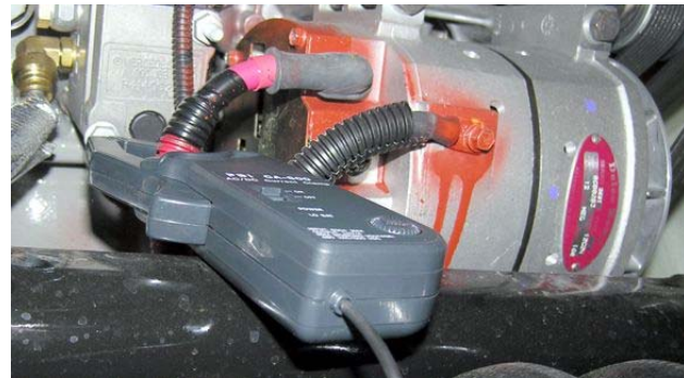
Fig. 13, Use an amp clamp around the positive alternator cable to measure the draw of the carbon pile.
