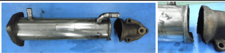
Cracked EGR Cooler from 7.8L 6HK1
