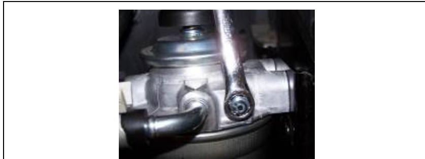
Figure 8 – Prepping Air Bleed Plug to Bleed System
