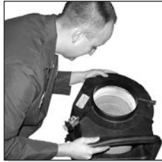
Inspect the engine air cleaner.
