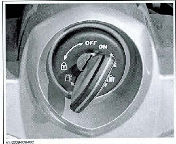
rmr2008-039-002 TYPICAL - IGNITION KEY ON
