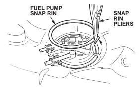
14. Remove the fuel pump assembly. To prevent damage to the float arm, lift the assembly straight up, and rotate it to the right.
