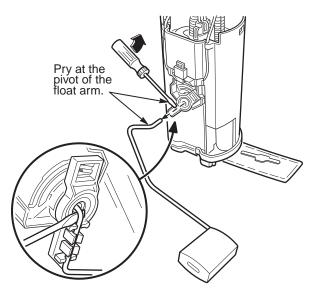
16. Remove the sending unit from the fuel pump assembly:
