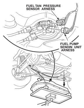
11. Use brake cleaner and compressed air to thoroughly clean the fuel pump and surrounding area.
