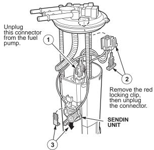
Remove the black locking clip, then remove the sending unit from the housing.
