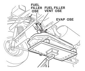
8. At the front of the tank, disconnect the fuel feed hose and the fuel return hose where they connect to the fuel filter and the fuel line. Remove the hoses from the support clip. Plug the hoses, and cap the lines to prevent any fuel leakage.
