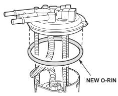
18. Of the two sending units in the kit, select the one with the connector that matches the connector from the original sending unit.
