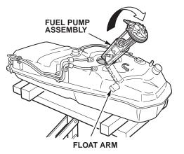
15. Insert a small screwdriver under the float arm at the brass bushing, and carefully pry the float arm out of the sending unit. Do *not* bend the arm.
