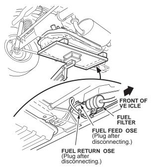
9. Remove the nuts and bolts from the corners of the tank. Do not remove the bolts from the skid plate.
