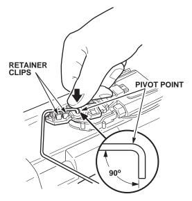
21. Move the float arm to its lowest position, then connect a DVOM to the sending unit, and measure the resistance. Resistance should be about 290 ohms. If the resistance is about 120 ohms, you have reinstalled the original sending unit.
