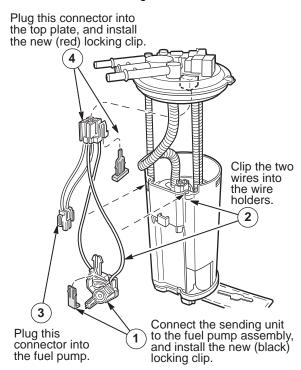
20. Reinstall the original float arm by pushing on its pivot point to snap it into place. After installation, make sure the arm moves freely under its own weight. If it does *not*, the pivot arm is bent, and the sending unit will *not* show the correct fuel level. To repair a bent pivot point, remove the arm, bend the pivot point back to its original 90-degree position, and reinstall the arm.
