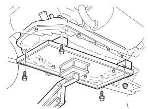
10. Partially lower the tank, then unplug the fuel pump/ sending unit harness and the fuel tank pressure sensor harness.
