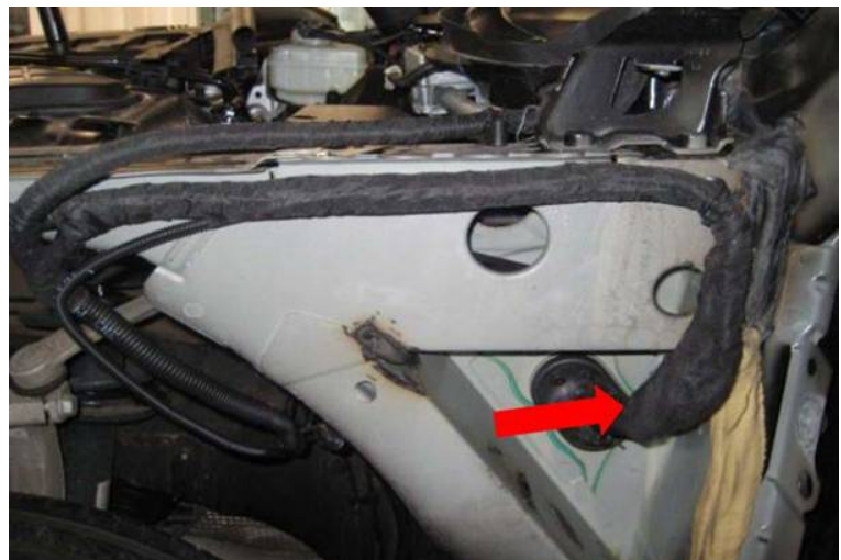
Figure 1. Left front fender is removed to show the left bulkhead grommet
