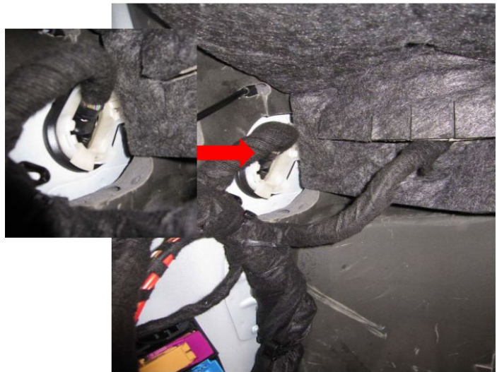
Figure 4. Grommet position photo, taken from inside the passenger compartment.
