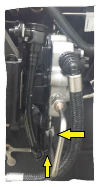
Example of a good OBFCT after the AFI Fuel Supply Line was repaired
