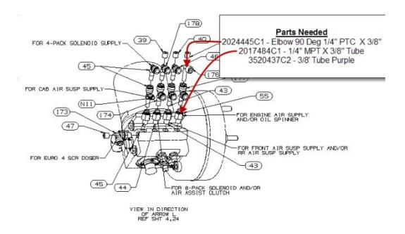
All other dryers air supplied to engine from secondary air tank pressure protected valve - Cummins ISX with SCR
