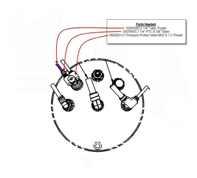
Parts and Routing information for missing engine supply line and fitting - Cummins ISX with SCR
