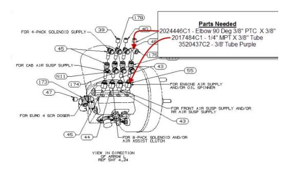
All other dryers air supplied to engine from secondary air tank pressure protected valve - N13 with SCR
