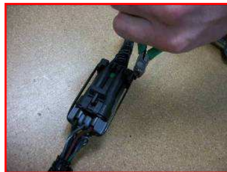
Fig. 6b: Zip Tie Secured and Trim
