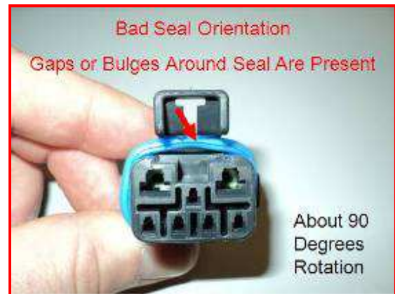
Fig. 4b: Improper Orientation
