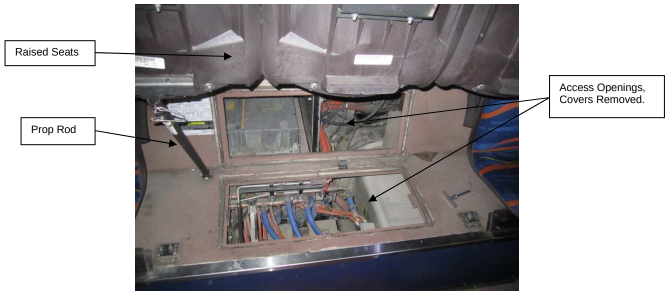
Figure 1: Access Openings Under Chesterfield Seats.
