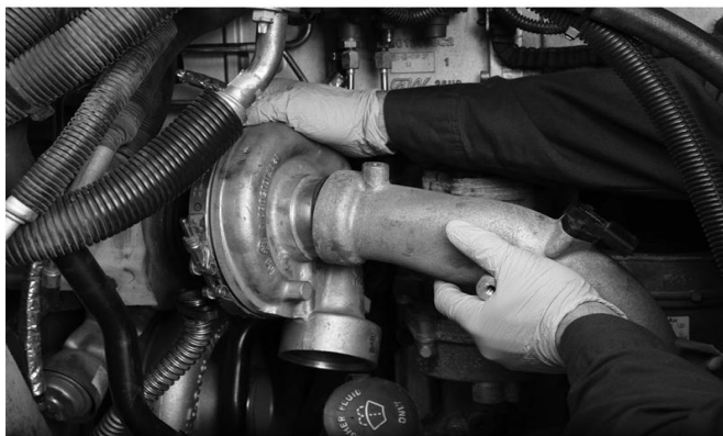
Figure 7. HP Turbocharger and Air Supply Duct.
