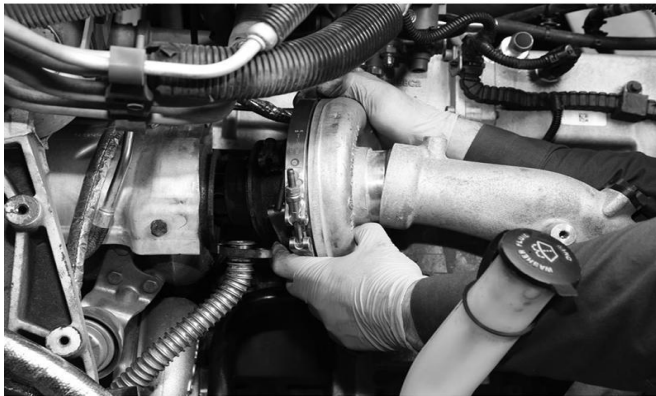
Figure 4. HP Turbocharger Removal.
