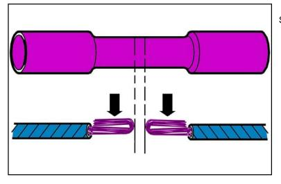
Splice the wires as shown.
