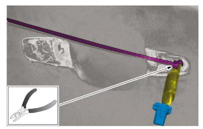
Complete the splices according to VIDA Repair->Cleaning, Inspection and Adjustment->371 Joining Cables
