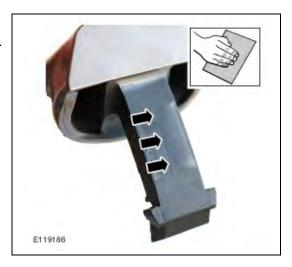
6. **LH and RH**: Using suitable 800-grit abrasive cloth, remove the molding split line from both rear edges of the door handle strap.
