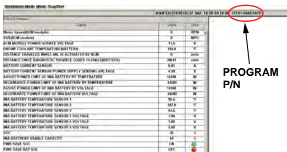
IMA System Data List Screen on the HDS (Example shown for a 2006-08 Civic Hybrid):
