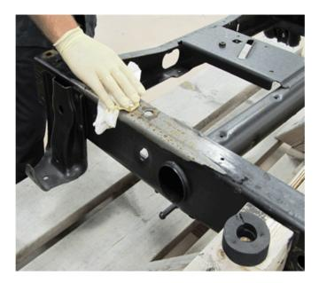
Using Lloyd's Pure Prep<sup>™</sup> Metal Surface Preparation P/N 25418 (10 fluid ounce bottle), or equivalent, saturate a towel or Scotch-Brite<sup>™</sup> (3M) pad with the pre-diluted solution and scrub the area well, rendering a foaming of the Pure Prep.<sup>™</sup> This will greatly improve adhesion and corrosion resistance in the repair areas.
