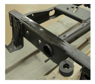
11. Apply a light flash-coat of Lloyds Kryptonite Metal Treatment P/N 36502 Life Long Rust Protection (14 ounce aerosol), or equivalent, to all rusted and bare areas of the frame where the wax coating was removed. This first coat should flash in approximately 3-5 minutes.
