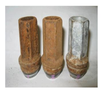
When removing wheel nuts with stainless steel caps, using a shallow socket may crack the cap causing corrosion underneath the cap and nut.
