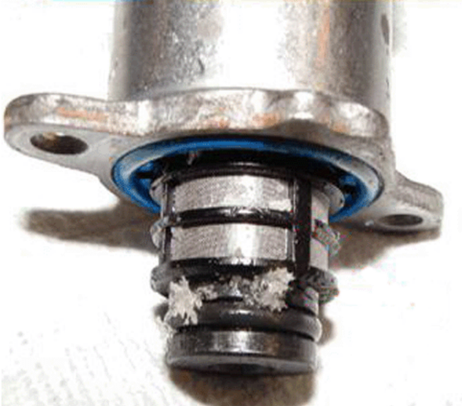
Fuel Pressure Regulator 1 Contaminated With Diesel Exhaust Fluid (DEF)
