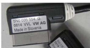
The cable above is the incorrect cable. This can be identified by the white collar around the cable.
