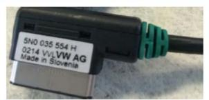
These 2 cables are the correct cables. Look for the green and blue collars around the cable.
