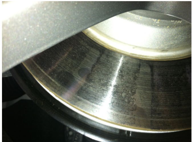
Figure 3. Discoloration on the brake disc due to chemical contamination from cleaner that was sprayed directly onto the disc.
