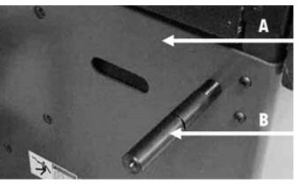
Figure 5. Back of balancer (A), calibration weight (B)
