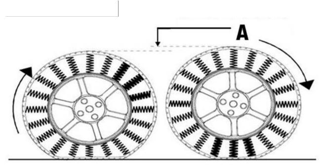
Figure 1. Vibration source from radial force variation (A).
