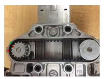
Figure 9. Installation of gear belt.
