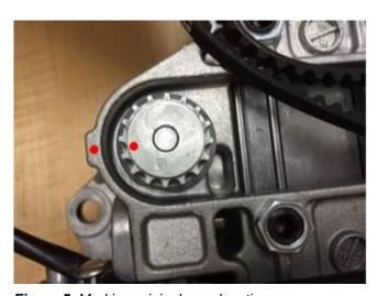
Figure 5. Marking original gear location.
