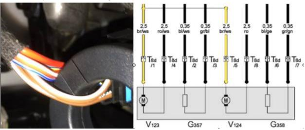
Figure 1. Current clamp installed (left), pins 1 and 5 (right).
