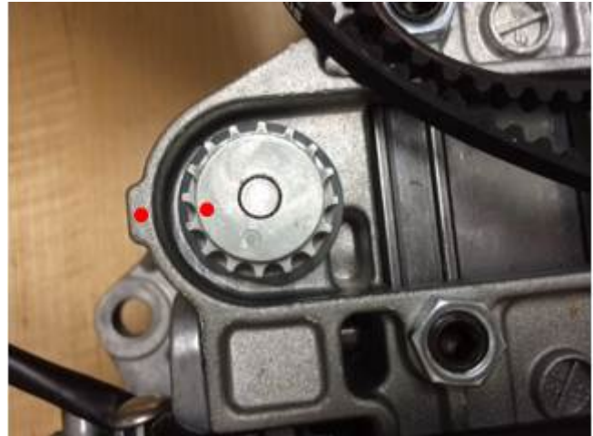
Figure 5. Marking original gear location.
