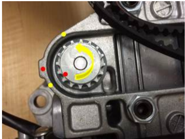
Figure 7. Marking the location with the greatest resistance in the counter-clockwise direction.
