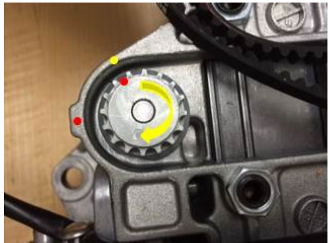
Figure 6. Marking the location with the greatest resistance in the clockwise direction.
