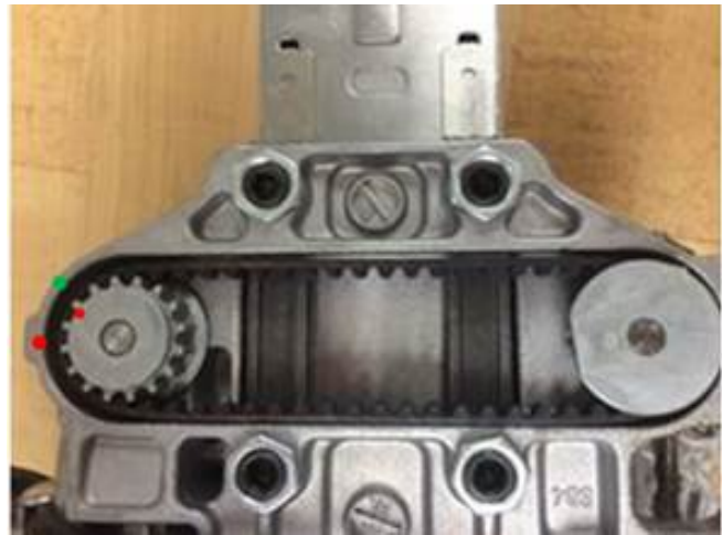
Figure 9. Installation of gear belt.
