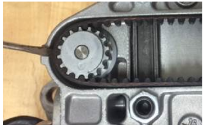
Figure 4. Remove the gear belt with a fine screwdriver.
