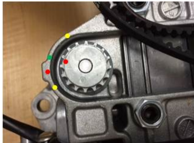
Figure 8. Placing a green dot in between the two yellow dots and turning the gear (red dot) to match the green dot on the housing.
