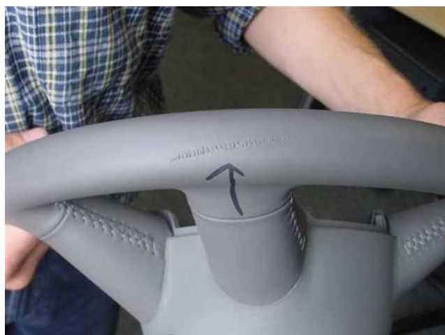
Figure 1. Example of damage from external impact.
