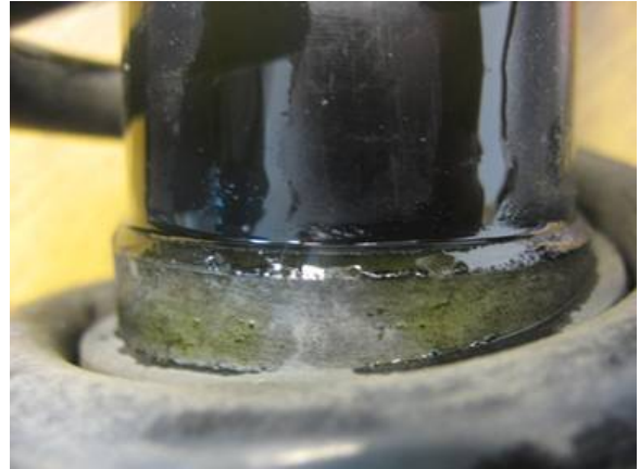
Figure 1. A leaking shock absorber.
