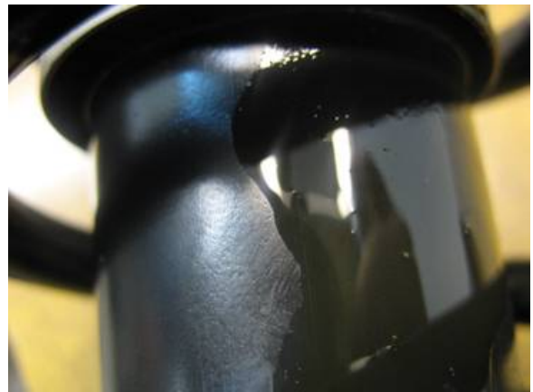
Figure 2. A leaking shock absorber.
