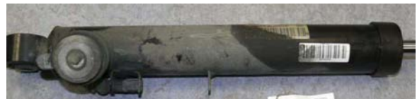
Figure 4. A shock absorber that is not leaking.
