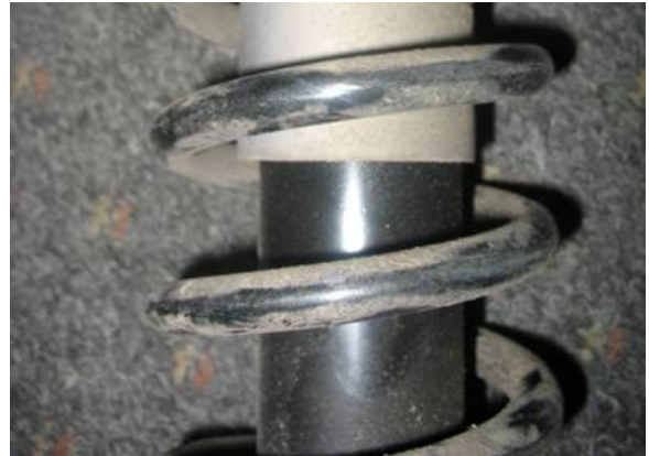
Figure 3. A shock absorber that is not leaking.
