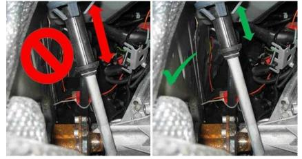
**Figure 1.** An incorrectly-fitted plastic sleeve (left) can be pulled down by hand. A correctly-fitted plastic sleeve (right) will stay in place when pulled.
