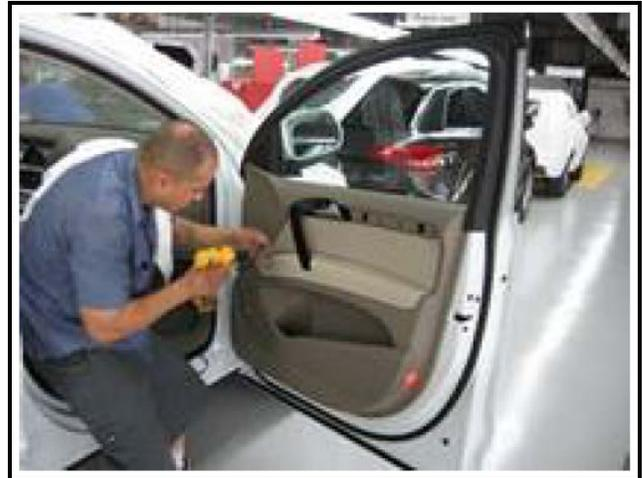
2. Carefully unclip the inner door panel cover.
