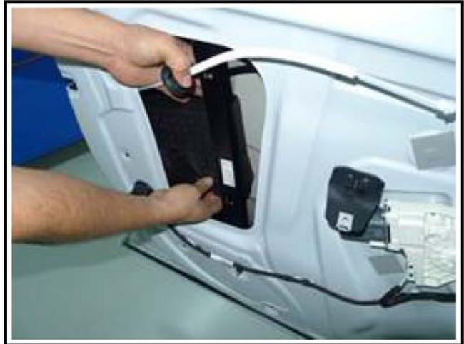
11. Using the mark that was previously made on the inside of the door skin as a guide, install the lower pad. The legs should rest on the top of the impact beam. Press the pad against the door skin so that the butyl strips stick the pad securely to the door skin. Slide the bracket along the impact beam if necessary such that the bracket correctly engages the slot in the pad.
