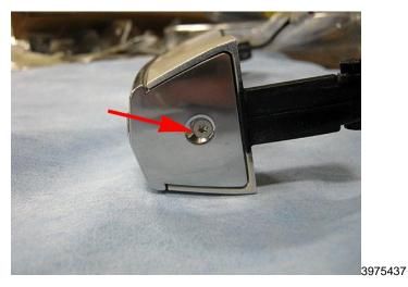
3. Remove the fastener at the rear of the handle.
